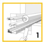
1.Clean the installations from dust, dirt and grease.
